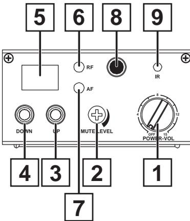
**A1** - Volume control fader for the HF module. From OFF to full power (clockwise).
