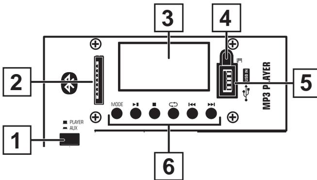
**B1** - Channel 1 input selector. Allows you to decide if the player or the Aux input will be active on channel 1 of the mixer.
