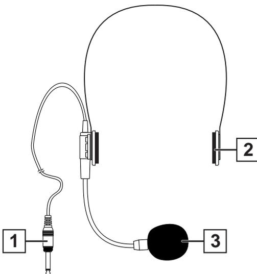
1 - Connector to plug the bodypack transmitter. Plug the headband microphone into the Jack #1 socket of the transmitter.
