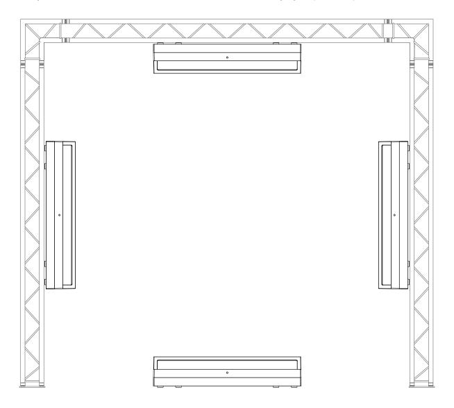
The Elumen8 Virtuoso 700 CYC IP RGBALC can be operated in a number of mounting positions as shown in the diagram above, hanging upside-down from the ceiling or truss, mounting sideways on truss or stood upright on a flat level surface. Always use a safety wire as an extra safety precaution to prevent damage/injury in the event a clamp fails (see the next page for clamp installation). Never use the carry handles for secondary attachments.
