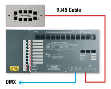
• If used with other equipment an AS180 PSU should be used to supply power to the Anyscene and then provide connection to the wider DMX network as follows,
