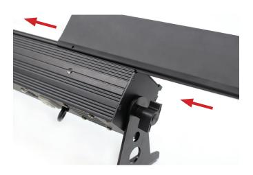
3) Carefully slide the eyebrow through the groove until the cutout holes for the thumbscrews line up with the threaded holes.
