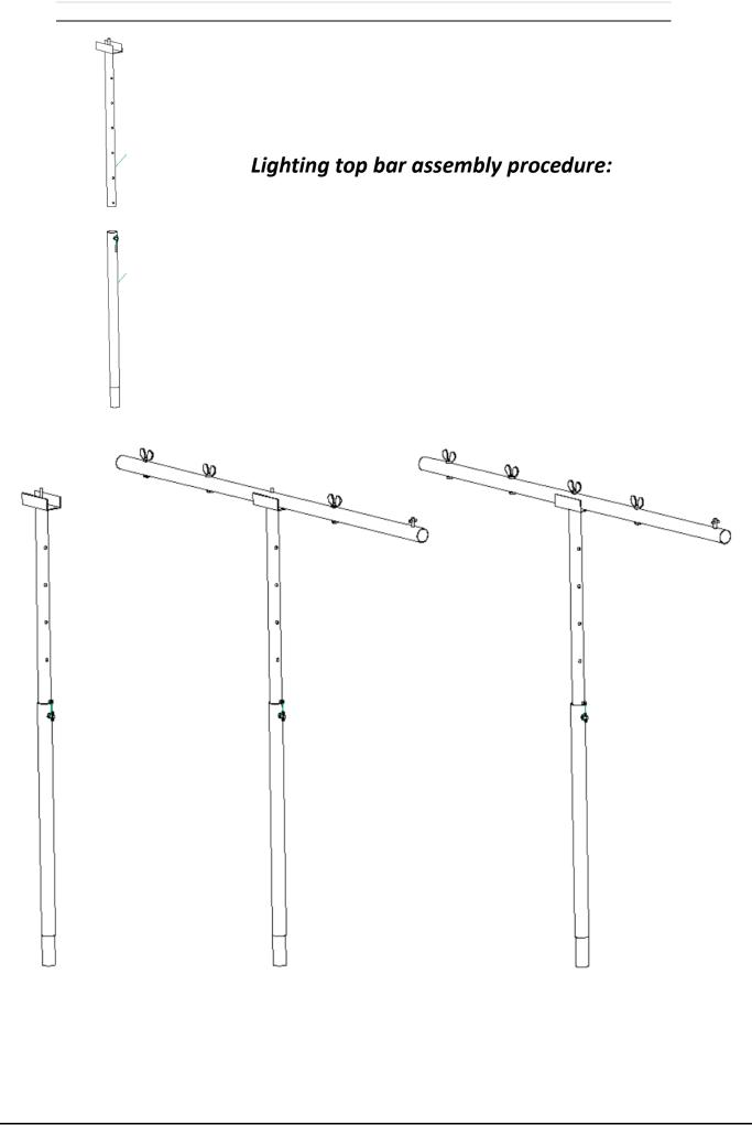
6. Insert tubes F into tubes E then set both tubes at the same height. Once the height has been determined, then insert the pins into the top of tube E – you are now choosing the height of the overhead bar that you will be using.
