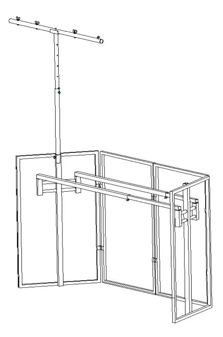
7. Add the "T" bar - tube G, onto the top of tube F and tighten the nut at the top.
