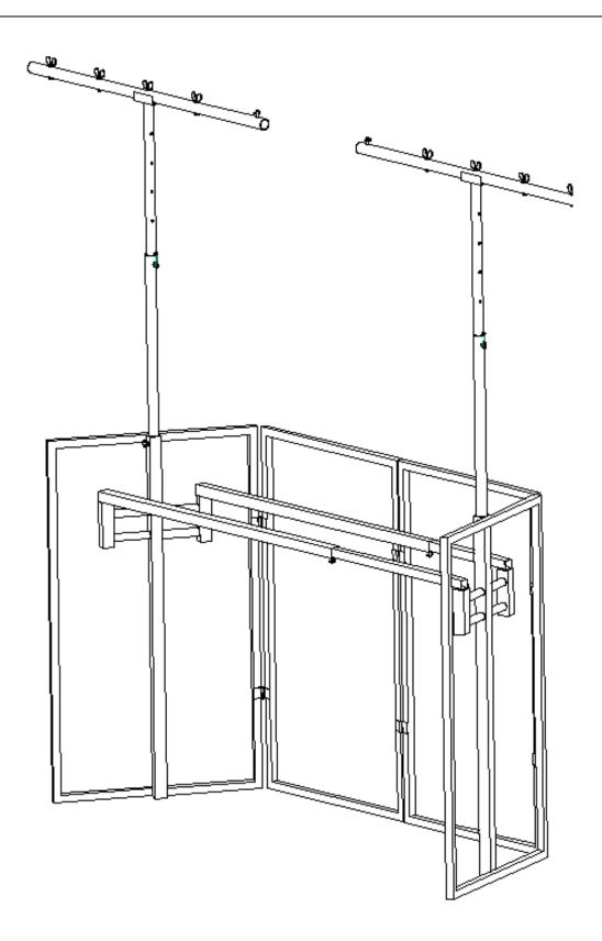
8. Insert each end of lighting gantry joining tube H into the ends of both tubes G and tighten the bolts. If you don't want to use joining tube H you can use both G lighting bars at different heights if needed and create 2 x "T" bar setups.
