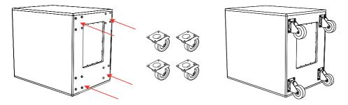
All holes comes with M8 drive-in nut. We suggest to use M8 x 30mm (at least) screws, hexagonal head with washer.
