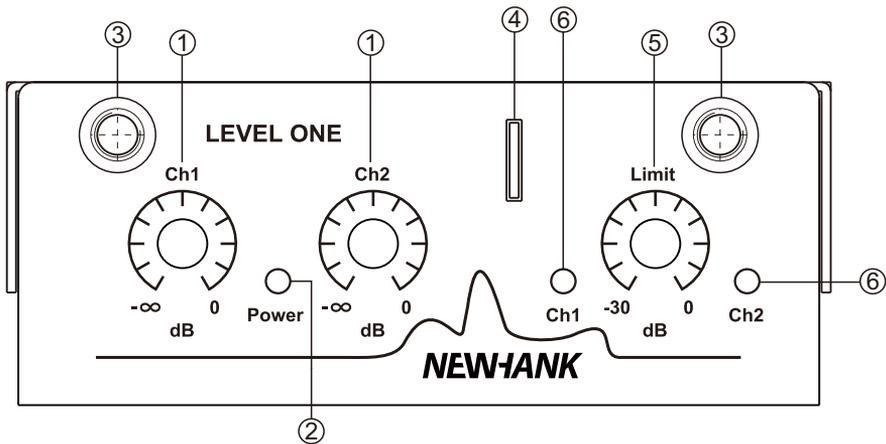
The front panel of the Level One contains all the controls and indicators and mechanical parts to lock the housing
