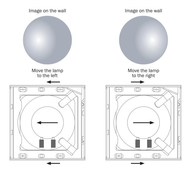
Please note: The adjusted hotspot may move during the first 100 hours of lamp operation as the lamp stabilises whilst its burning. Please adjust the lamp if the hotspot moves out of the centre.
