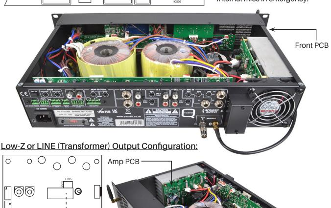
The unit is pre-set by the factory to high-voltage line (100V) output operation. To convert the amplifier to low-impedance (4-8 Ohm) operation, the plug connected to the toroidal transformer, nearer the fan side of the unit, should be unplugged from CN5 on the amplifier PCB (a short pair of heavy red and black wires), and replaced by the spare plug connected to the low impedance output socket (same wire types to a 2-pin 5mm-pitch screw terminal type: CN7).
