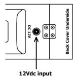
Alternatively, the L25 can be powered by an external 12Vdc source (such as car battery) connected via a 2.1mm DC jack located between the pistol grip and rear cover hinge (a lead is supplied for connection to a car cigar lighter socket). This jack is covered with a rubber plug for protection.
