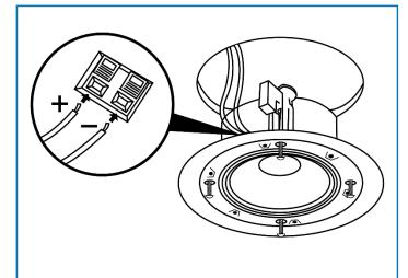
Take the speaker unit out of the packaging and remove the grille. Connect the speaker wires to the appropriate "+" and "-" connections (select the desired tappings for 100V units).
