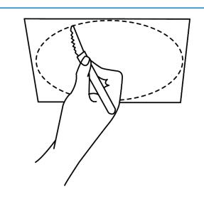
Cut out the trced area using a pad saw or other suitable tool.
