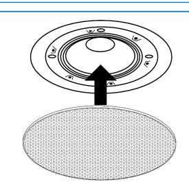
5. Place the speaker grille back onto the speaker, it will fix magnetically.
