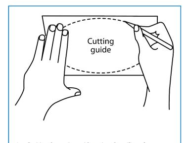
Position the cutting guide against the ceiling where you intend to install the speaker and trace around it.
