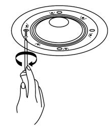
Once in place, turn the 4 fixing screws clockwise. This will
