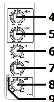
6. FX This control regulates the amount of the channel signal that is fed to the digital delay effects section, varying the amount of delay effect (see Digital Delay below)
