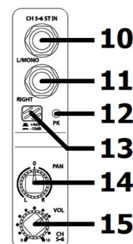
13. Level switch Sets the line input level to  $-10\text{dB}$  if pressed in or  $+4\text{dB}$  if not pressed in.
