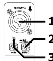
2. IMPED switch Press this button in to set the input impedance to instrument level or leave the button in the up position for a line level input. (instrument level is usually for pickups, such as those on a guitar. Electronic keyboards usually produce a line level output)
