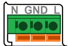
Feed the wiring carefully into the wall cavity to take up any excess, rather than compressing it inside the back box, which may damage the wire and connections. Push the WA-215 unit firmly onto its mounting plate to fix into the back box or wall cavity. Keep the mains power isolated (off) until the WA-215 is fully installed into the wall, covering the rear panel wiring.
