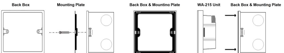
Alternatively, the mounting plate can be fitted into a standard 86 x 86mm pattress box top accommodate the WA-215, so long as there is a minimum 47mm mounting depth
