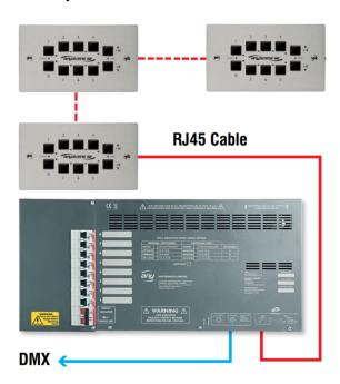
• If used with other equipment an AS180 PSU should be used to supply power to the Anyscene and then provide connection to the wider DMX network as follows,
