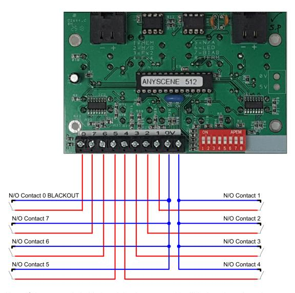
Note: If the contact is held closed the Anyscene 512 will lock to the selected scene until the contact is reopened.
