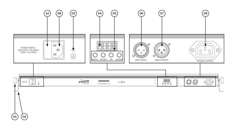
01 - Bracket tightening knobs
