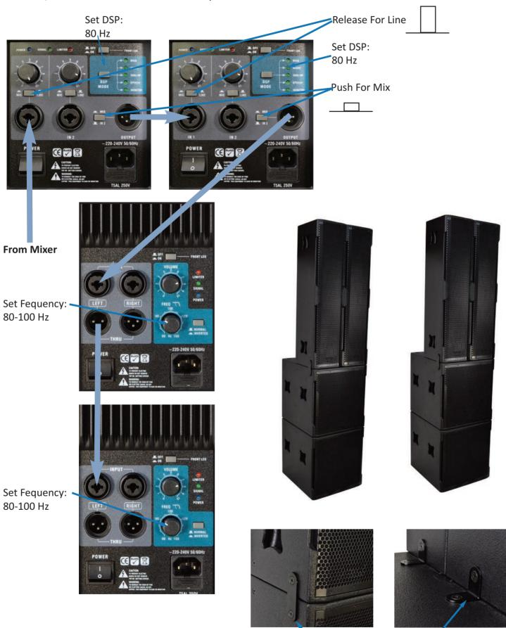
Make sure the speaker interconnecting plates are securely fitted, this is essential for safety reasons.
