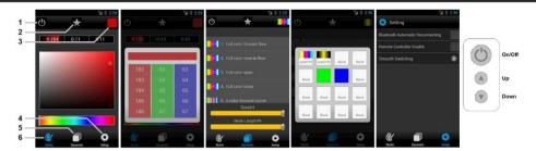
The Color Stream application has 3 edit screens for Static (6), Dynamic (5) and Setup (4) menus.
