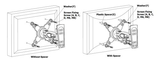
For VESA sizes bigger than 100x100, the supplied adaptors may be used. Attach the VESA extension arms as shown below using M5 12mm screws and nuts supplied.
