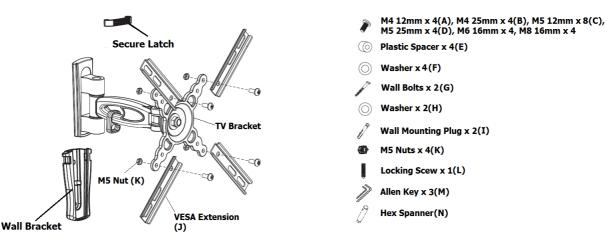
For this installation you will also require a pencil, tape measurer, electric drill, stud finder and a Philips (cross) screw driver.
