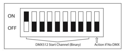
Normal DIP Switch assignments: DMX start channel = 1
