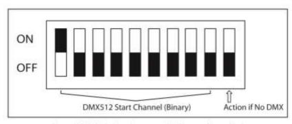
Normal DIP Switch assignments: DMX start channel = 1
