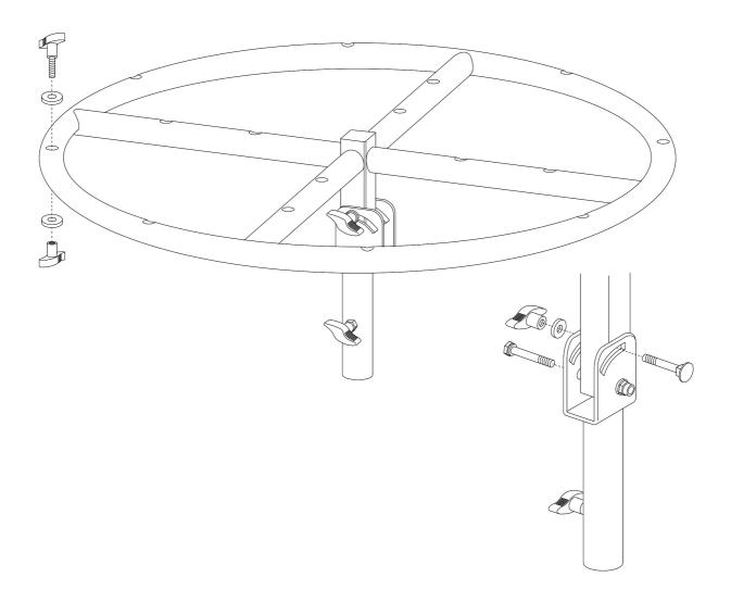
The Novopro LIBRA1 round lighting bracket has been designed for ease of use as well as safety. The bracket has a standard 35mm pole mount for all standard lighting stands (not supplied).
