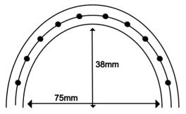
A curve of less than 75mm may stress the PVC sheath and lead to product damage and electrical failure.
