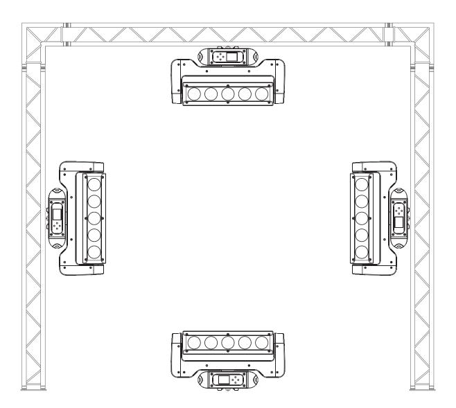
The Equinox Switchblade can be operated in a number of mounting positions as shown in the diagram above, hanging upside-down from the ceiling or truss, mounting sideways on truss or stood upright on a flat level surface. Always use a safety wire as an extra safety precaution to prevent damage/injury in the event a clamp fails (see the next page for clamp installation).
