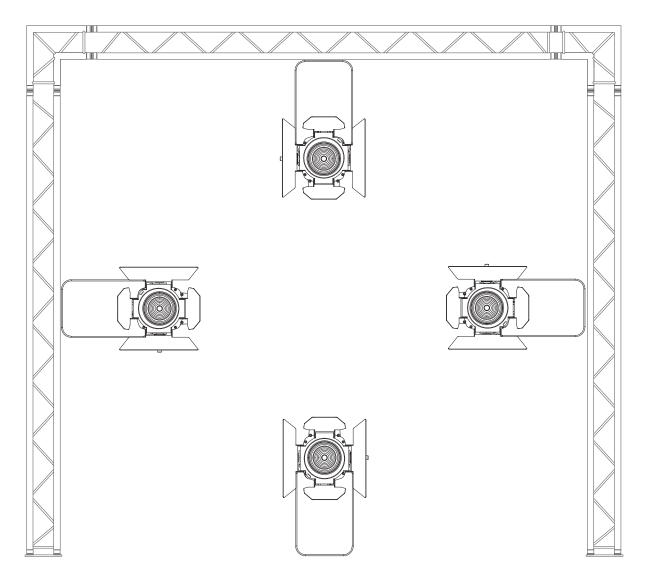
The Libretto Mini RGBAL Fresnel can be operated in a number of mounting positions as shown in the diagram above, hanging upside-down from the ceiling or truss, mounting sideways on truss or stood upright on a flat level surface. Always use a safety wire as an
