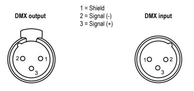
Connect the DMX output of the first unit in a DMX chain with the DMX input of the next unit in the chain. Always connect the the output of one unit with the input of the next unit until all units are connected.
