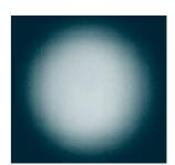
The PC beam is well defined with little light scatter, similar to a profile beam with 114 Hamburg Frost.
