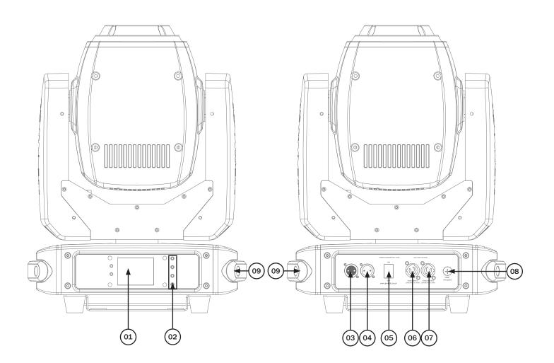
01 - LCD display 02 - Function buttons 03 - 3-Pin DMX input 04 - 3-Pin DMX output 05 - Power switch
