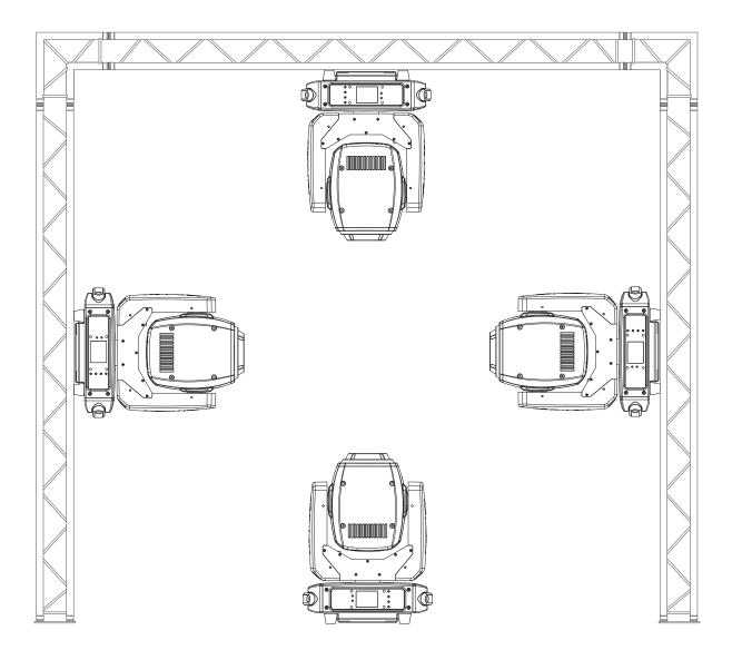
The Equinox Fusion 150 Spot can be operated in a number of mounting positions as shown in the diagram above, hanging upside-down from the ceiling or truss, mounting sideways on truss or stood upright on a flat level surface. Always use a safety wire as an extra safety precaution to prevent damage/injury in the event a clamp fails (see the next page for clamp installation). Never use the carry handles for secondary attachments.
