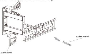
**STEP 4** – Install TV on to the wall bracket.
