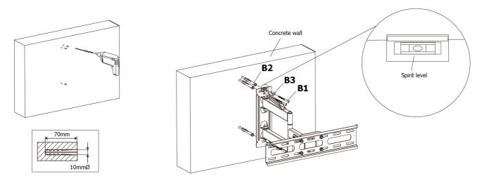
For plaster wall installation first of all find out where the wood stud is behind the wall using a stud finder. Then work out the height of the installation and ensure it is level using the spirit level. Use a pencil to mark where the mounting holes will be and use an electric drill to drill a hole that is around 5mm in diameter and 70mm deep. Install the wall bracket as follows.
