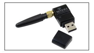
will scroll through the operating protocols. Once you have selected the chosen protocol, press and hold the button on the dongle for 3 seconds. The LED will illuminate white, then turn blue (transmit mode) or stay white (receive mode). The unit is now set in your chosen protocol.
