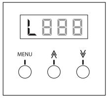
Press the "**MENU**" button to enter Dimmer limit mode. Use the "**UP**" or "**DOWN**" buttons to change the value between 10-100.
