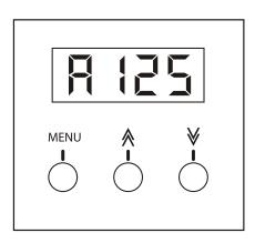
By using the "**UP**" or "**DOWN**" buttons the user is able to select the required DMX address. Once the DMX address is selected, it will be automatically stored into the units memory.
