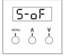
Press the "**MENU**" button to exit switch pack mode. In Switch pack on mode the output is on and the fixture will illuminate
