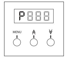
Use the "**UP**" or "**DOWN**" buttons to change the value between 00-100. Once the dimmer preset is selected it will be automatically stored into the units memory.
