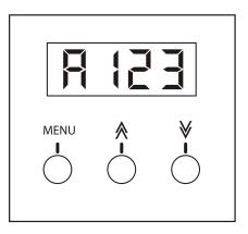
When the unit is powered up the unit will show the DMX address that the unit was last in before it was powered down. If the DMX address 123 was selected in the units last use the unit will display "A123".
