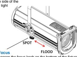
Loosen the focus knob on the bottom of the fixture, gently slide engine forward for flood and backwards for spot, tighten focus knob once focused.
