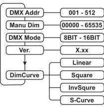
**Important:** if you don't confirm the dimmer value by pressing ENTER, the dimmer will (after 5secs) automatically return to the last setting.
